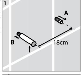
**2\_**Prepare the connection for the outlet pipe to the correct dimension shown. Assemble the outlet connection on the WC and cut it according to the correct length. Then locate the WC on the fitting bolts and push it to the wall taking care to correctly engage each connection. Applying a suitable silicone lubricant prior to final install will assist.
