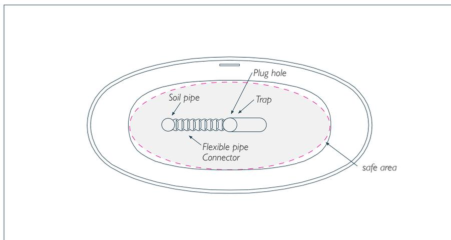
Remember you do not need to fit your bath directly over the soil pipe. It can be positioned anywhere within the shaded area.
