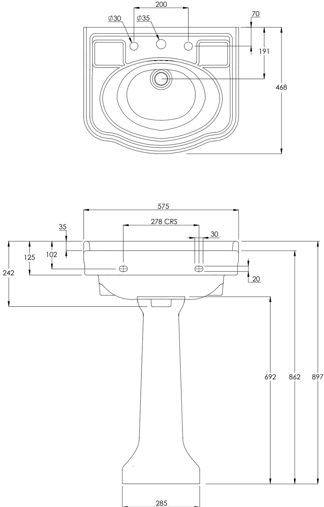
ALL SHOWN DIMENSIONS ARE IN MILLIMETERS AND ARE SUBJECT TO STANDARD CERAMIC TOLERANCES.
