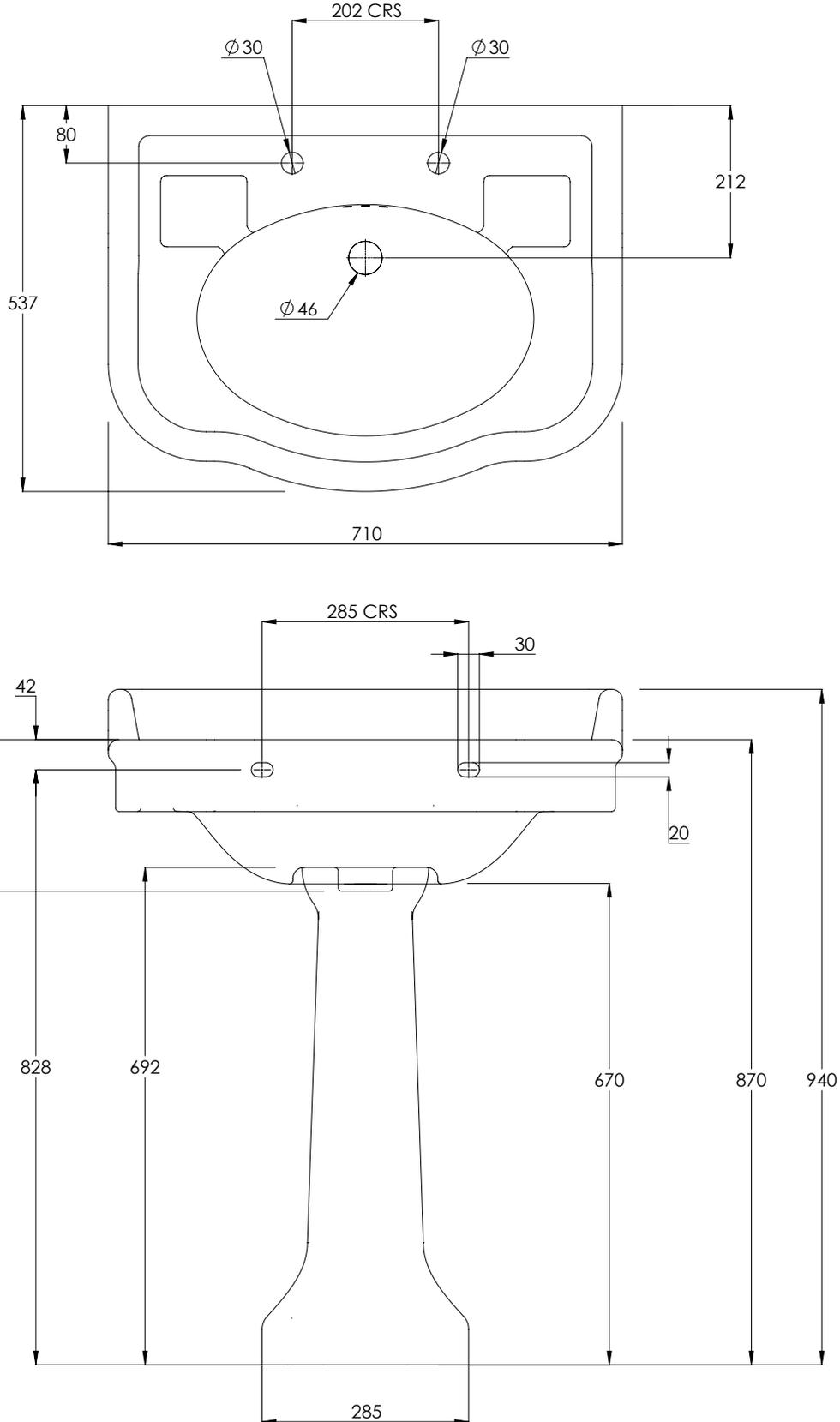
ALL SHOWN DIMENSIONS ARE IN MILLIMETERS AND ARE SUBJECT TO STANDARD CERAMIC TOLERANCES.
