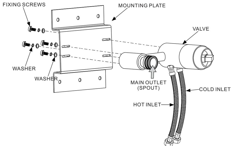
FIG. 1 INSTALLATION OF SPOUT
