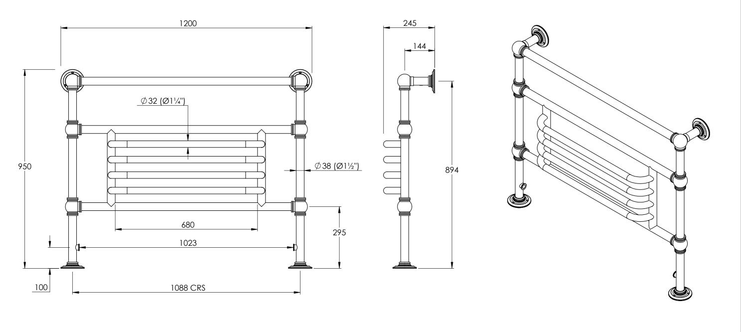
BTU/HR AT DELTA 60: TEST PRESSURE: 4176 CONNECTIONS: FI 1/2" BSP MAX WORKING PRESSURE MAX WORKING TEMPERATURE: HEAT OUTPUT DETERMINED IN ACCORDANCE WITH EN 442 BARD & BRAZIER LIMITED T: +44 (0) 121 270 2222 TITLE: MARSTON ROAD E: INFO@BARDBRAZIER.CO.UK BARONIAL GRILLE FLOOR MOUNTED TOWEL RAIL 950mm x 1200mm - HYDRONIC
