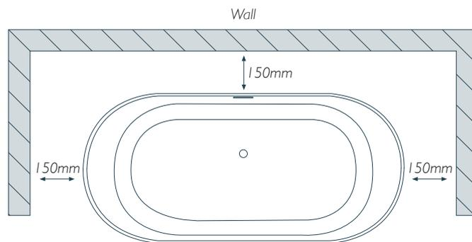
Locate the bath in its intended position and draw around the lower outer edge and mark the waste location with a pencil. Access to the waste and any isolation valves should be considered.
